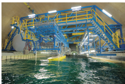
Ship model in the Depressurised Wave Basin
